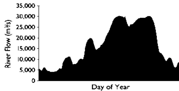
FIGURE 1-3. River Hydrographs from Around the World. Each of these four hydrographs portrays a river's flow variations over the course of a single year, which are influenced by different climates and watershed sizes. The Korean river is relatively small, and it rises quickly in response to seasonal rainstorms that occur midyear. The Brazilian river gathers rain-fed runoff from a larger watershed; its flow rises are more gradual and prolonged, and occur earlier in the year. The Yampa River in Colorado is fed by melting snows, producing a distinctive flood peak of long duration in late spring. The Mississippi River receives water from many large tributaries, and its flow increases slowly toward a midyear peak.
